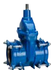
Series 01/70 Supa Plus™ gate valve Tensile coupling ends for PE and uPVC pipes Ductile iron DN40-300 PN16
