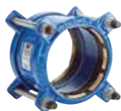
Series 621/10 Supa Plus™ straight coupling Tensile for PE and uPVC pipes Ductile iron DN32-300 PN16
